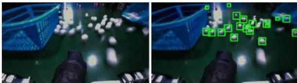
Fig. 5 A capture from processed image stream; Bouncing balls are recognized in green boxes.
